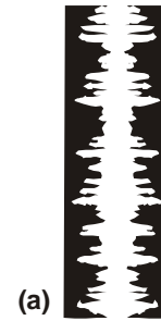
(a) Fig. Sound track on a film which varies the intensity of light reaching the photo cell.
