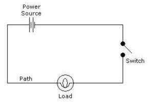
These diagrams are usually restricted to showing the power source, switches, loads (typically bulbs), and the path of the wiring. To answer these questions you need a basic understanding of how electricity flows around a circuit.
