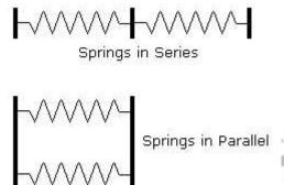
When springs are arranged in series, each spring is subjected to the force applied. When the springs are arranged in parallel the force is divided equally between the springs. Example Spring Question
