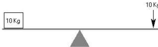
However, if you want to lift a weight that is heavier than the force applied you can move the fulcrum closer to the weight to be lifted. This affects the force required in the following way:
