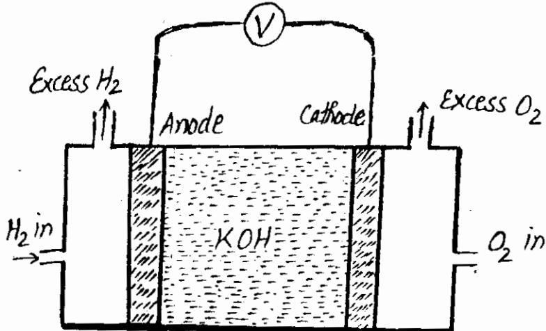
(Hydrogen - Oxygen fuel cell)
