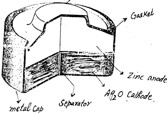
The Cathode is made of Silver Oxide,  $\text{Ag}_2\text{O}$  and anode is made of Zinc metal. The voltage of this battery is about (قریب) 1.5V. Here  $\text{NaOH}$  or  $\text{KOH}$  is used as an electrolyte. Following reactions occur in the battery.
