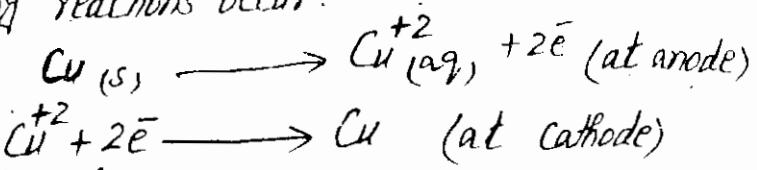
(VI) Electrolysis is used for Purification of copper. Anode is made of impure copper. The cathode is made of thin sheet of pure copper. The solution of  $\text{CuSO}_4$  is used as electrolyte. During electrolysis  $\text{Cu}^{+2}$  ions from anode go to solution and then pure Cu deposits on cathode. The impurities are left at anode.
