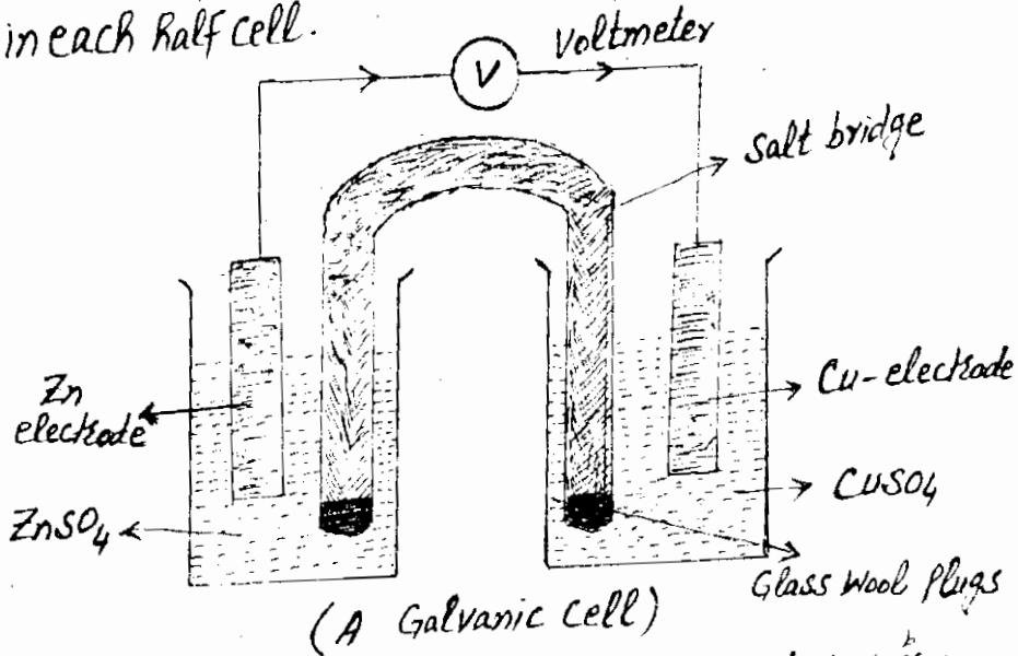
In left hand side cell a Zinc strip (S.) is dipped in 1M  $ZnSO_4$  solution. It acts as anode. In right hand side cell, a Copper strip is dipped in 1M  $CuSO_4$  solution. It acts as cathode. The two solutions are connected by a salt bridge.
