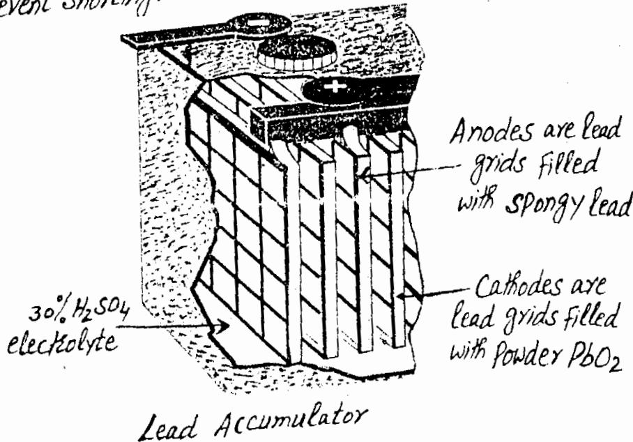
**Discharging:-** At the anode the lead atom loses two electrons and form  $Pb^{+2}$  ion.
