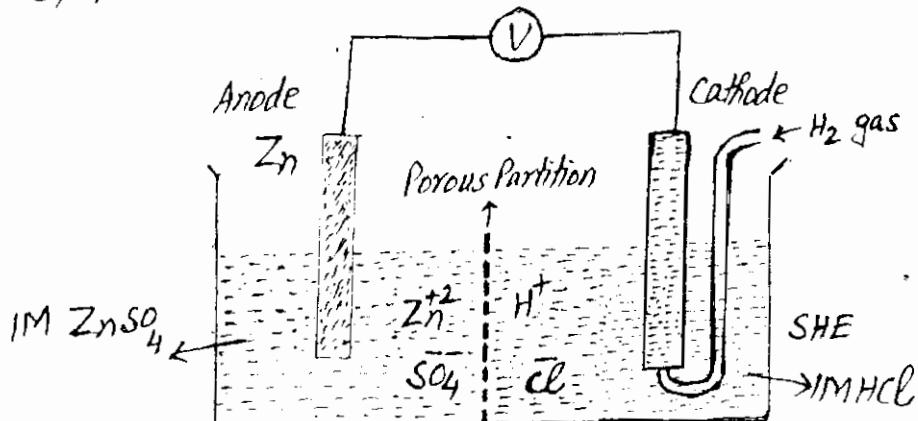
The reading on voltmeter gives electrode Potential of Zn. It is 0.76 Volts. It means that Zn has greater tendency to give up electrons than that of Hydrogen by 0.76 volts. In this arrangement Zn electrode acts as anode and SHE acts
